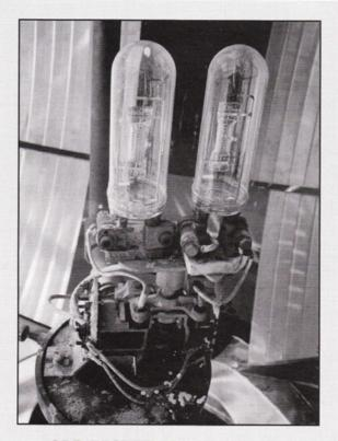
**OLD LIGHTING EQUIPMENT** The old lighting equipment with 1,000 watt bulbs is shown inside the lens. This assembly was removed and replaced with an all-new unit with larger bulbs.
