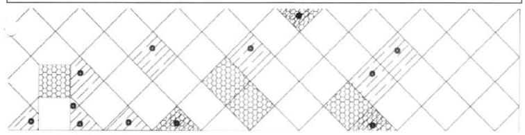
Legend: 1) Black dots/Slats are Broken Glass or Lexan. 2) Wire mesh Glass panels
