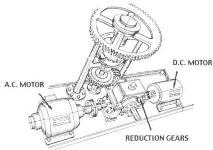
ELECTRIC LENS TURNING MECHANISM
