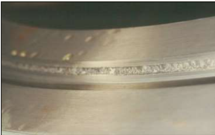
Failed Ball Bearing Track Source: Art Makenian
